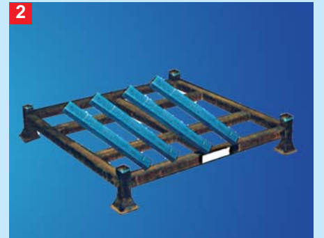
putting square pipe stays on Bottom plate in equal pitch pattern
